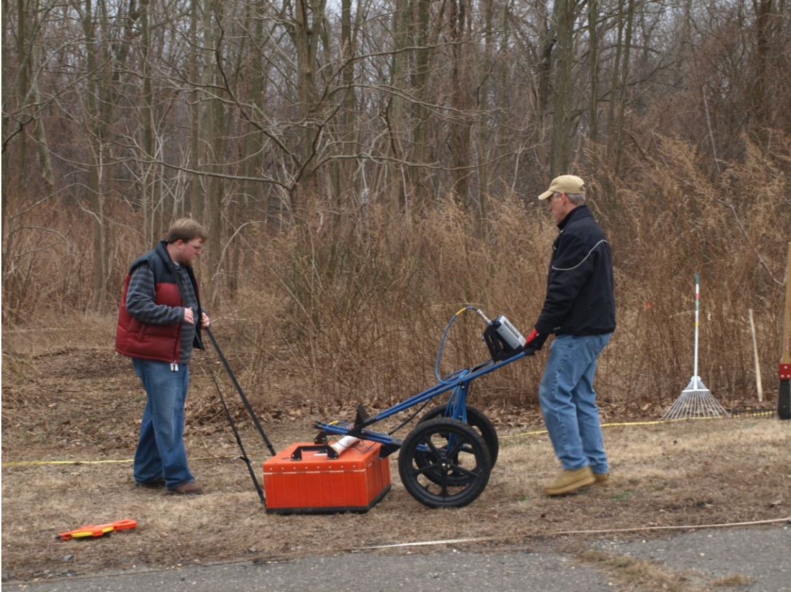
A second ground-penetrating radar unit being moved into position for another round of testing
