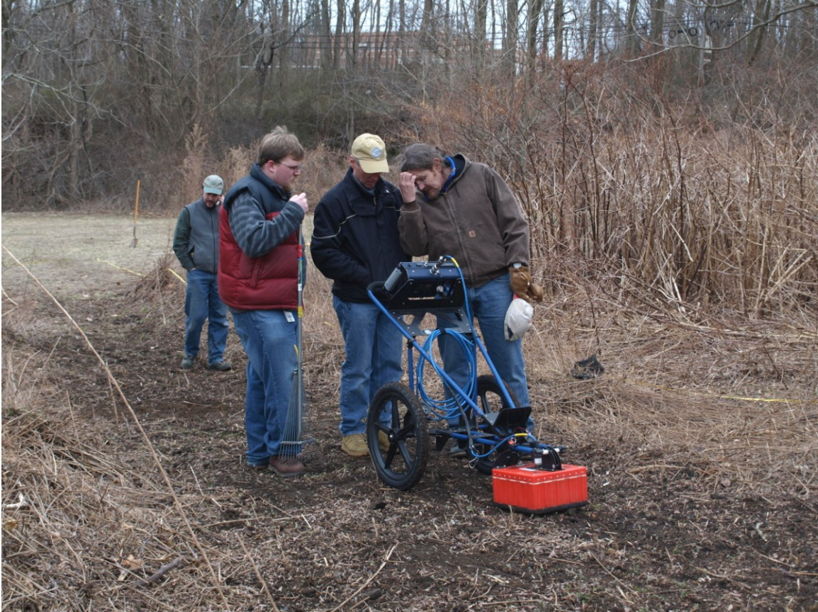
Researchers analyze the read-out from the ground-penetrating radar
